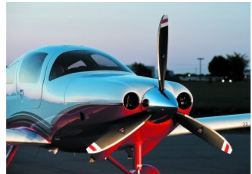
McCauley's new Black Mac Carbon composite prop on a Cessna 400.
