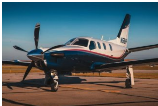
Five-blade Hartzell composite propeller on a TBM 900.
