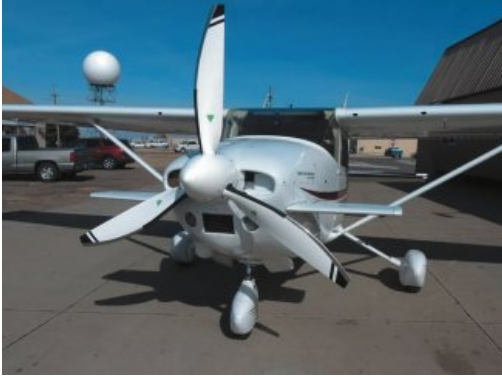
Three-blade MT composite prop on the King Katmai conversion of a Cessna 182.
