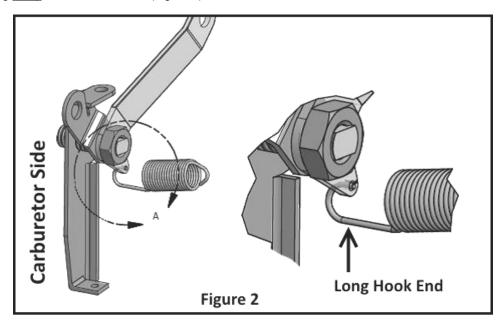
b. Using only your hand, grasp <u>ONLY</u> the bottom hook and attach it to the fixed linkage. The hook end should be facing <u>toward</u> the carburetor body as shown in Figure 3. <u>DO NOT TWIST the bottom hook</u> during installation; doing so may severely limit the longevity of the spring. Correct installation position is shown in Figure 4.
