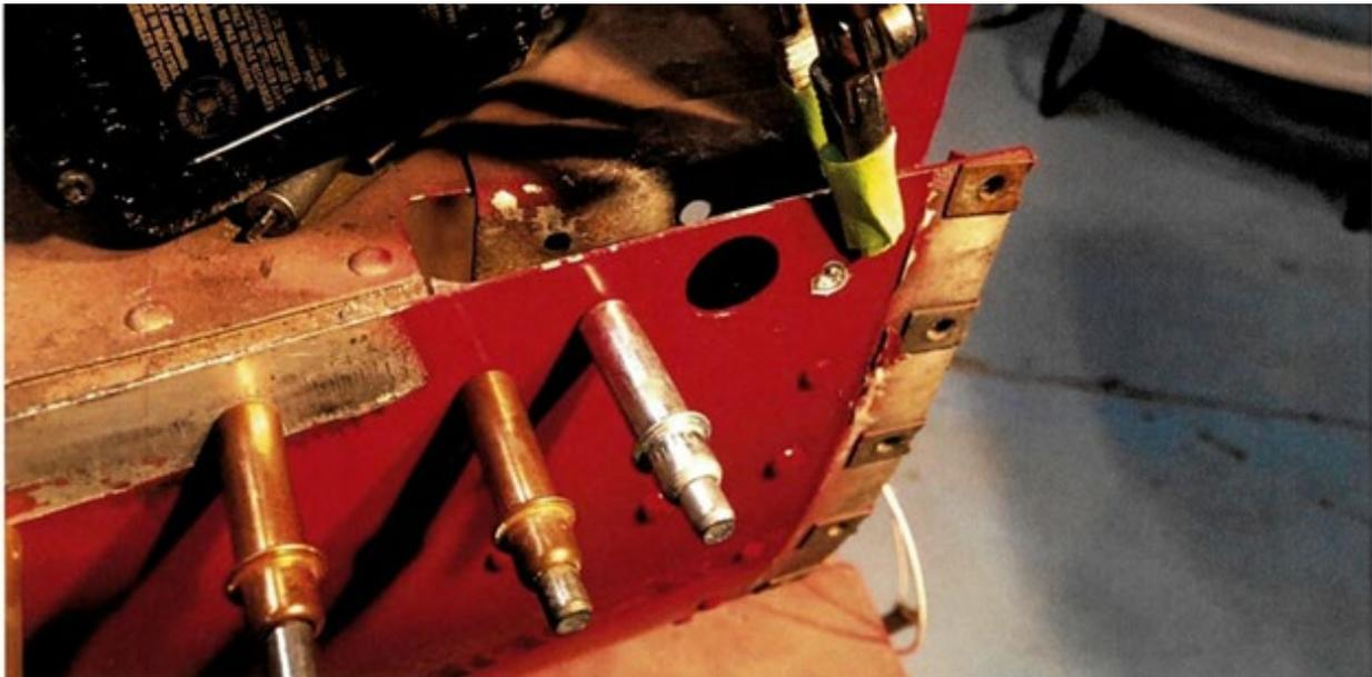
**Figure 19: Clamp aft end of Splice to aircraft**
