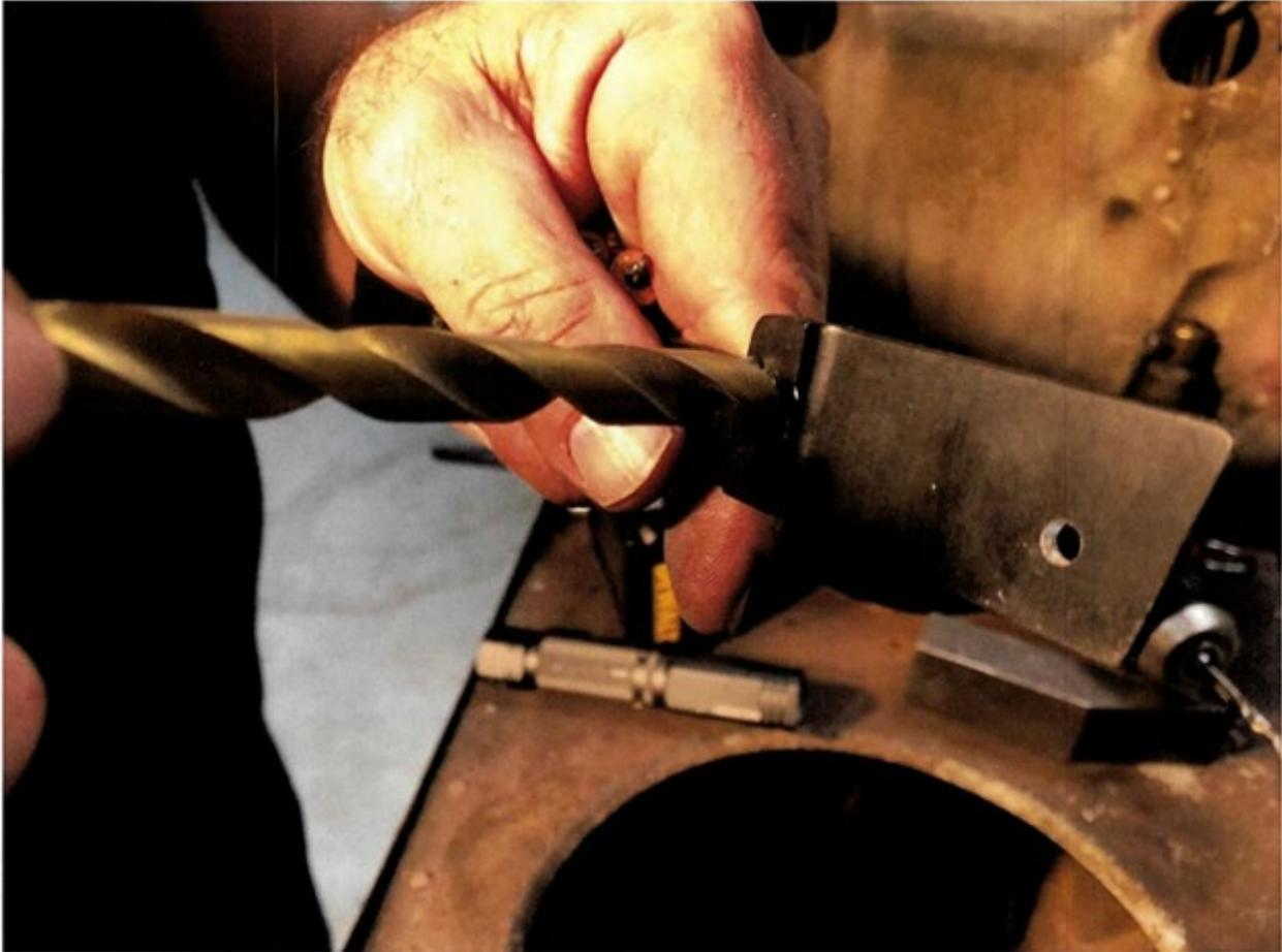
**Figure 25: Deburr Angle Splice Holes**
