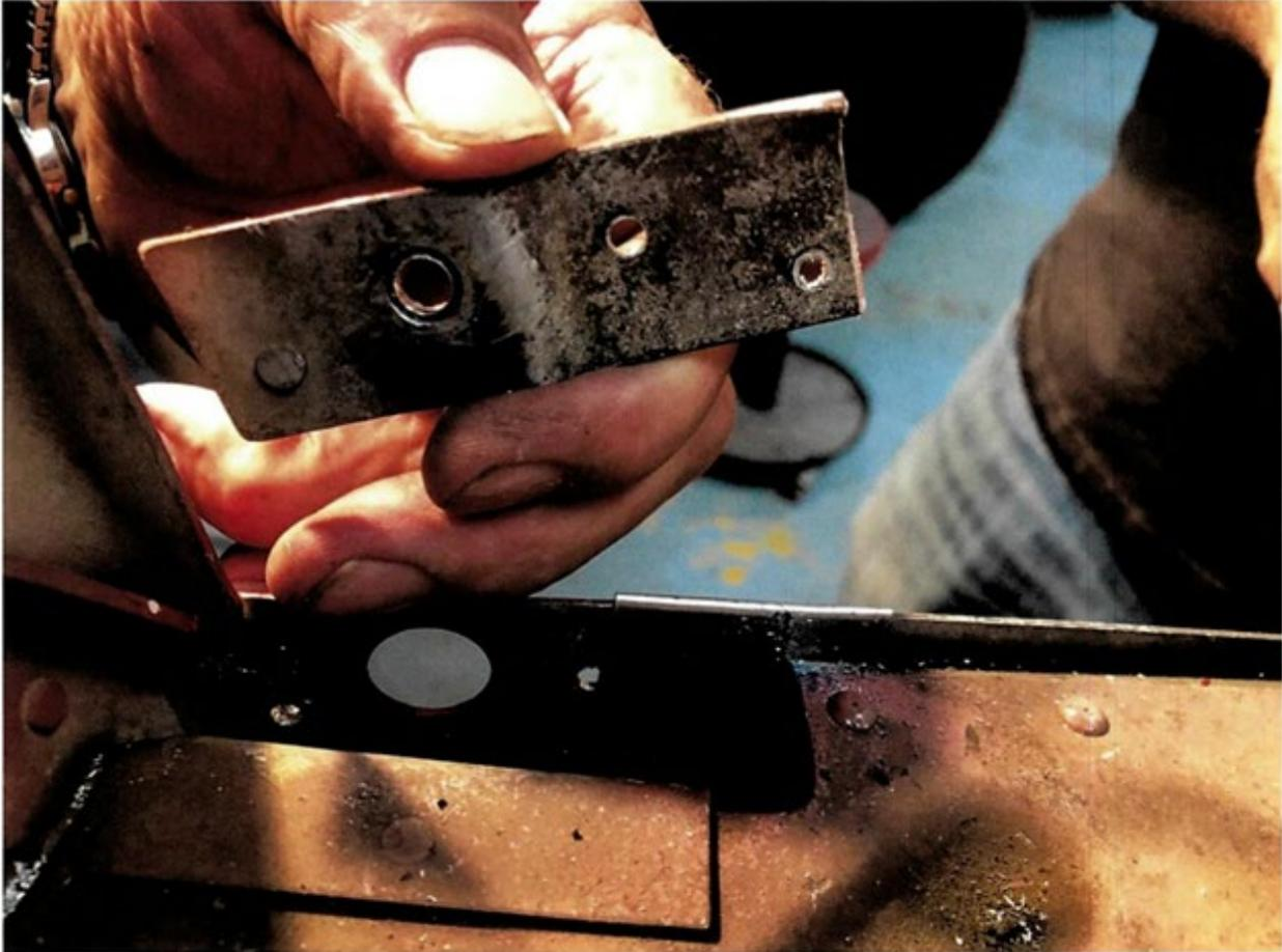
**Figure 12: Remove cut off portion of reinforcement angle**
