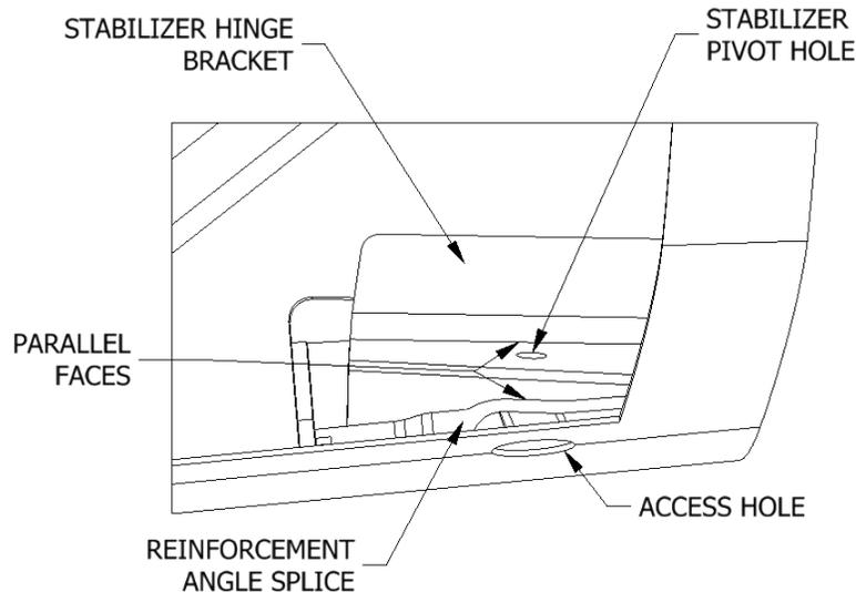
Figure 14: Reinforcement Splice Placement Diagram
