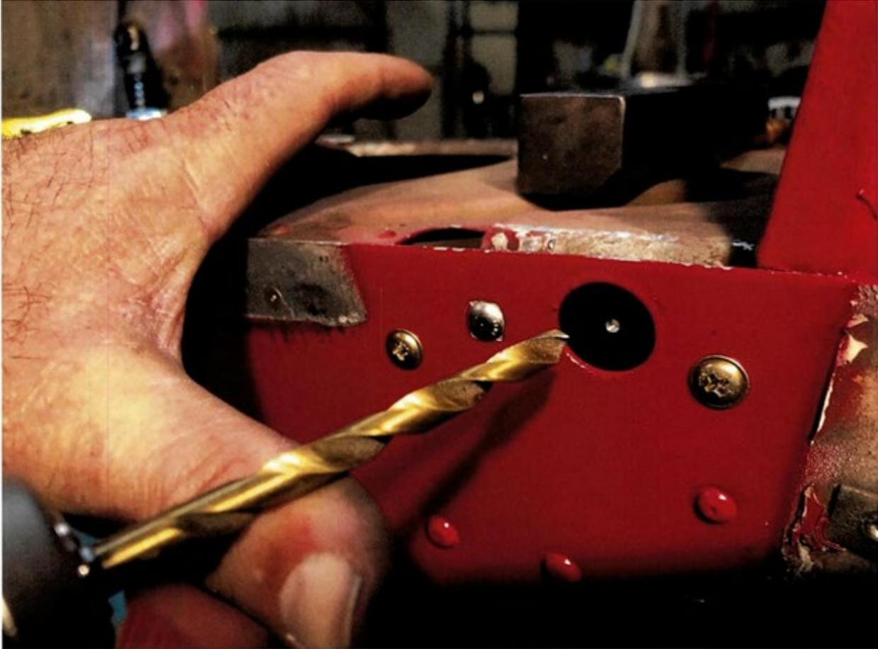
**Figure 32: Open up pilot hole**
