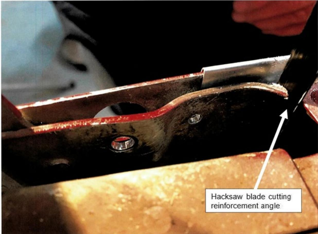
**Figure 11: Cutting Reinforcement Angle**
