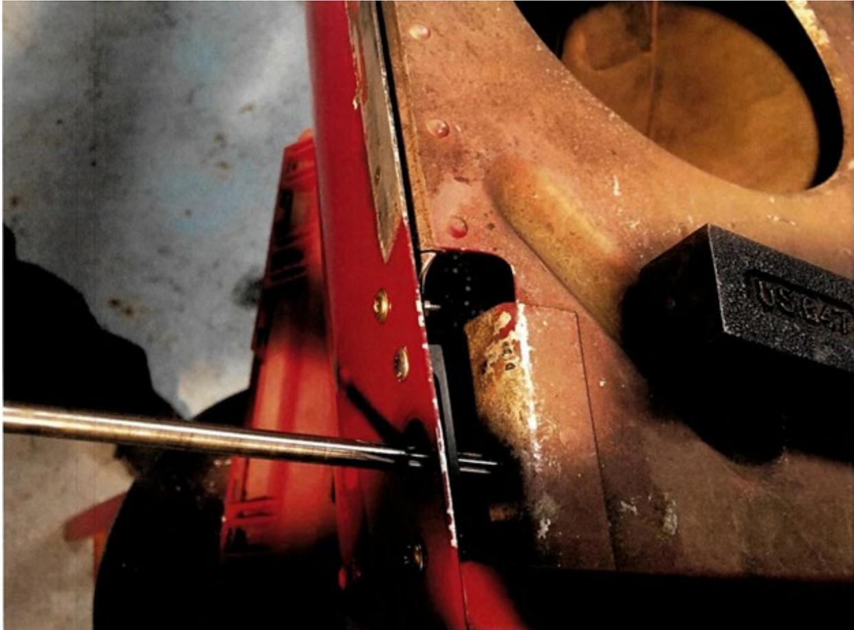
**Figure 34: Ream inboard stabilizer pivot hole**
