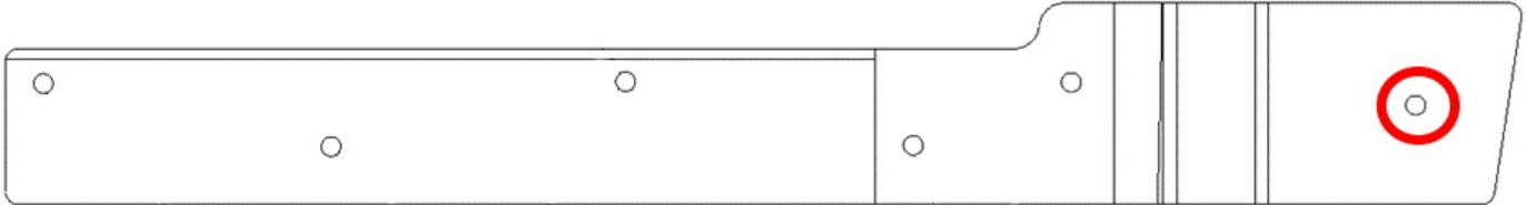
Figure 20: Match Drill Diagram – Most Aft Hole
