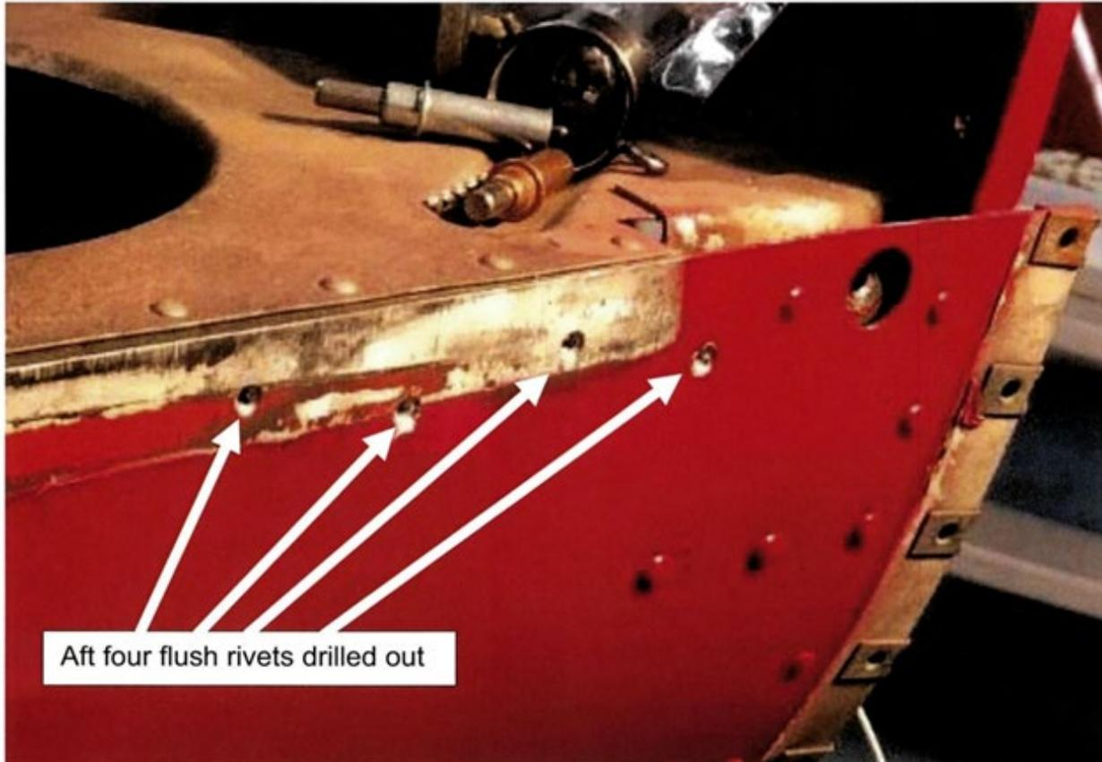
**Figure 8: Aft four AN426AD-4 rivets drilled out**
