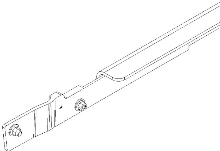
**Figure 5: Close up view of STC reinforcement angle splice part**
