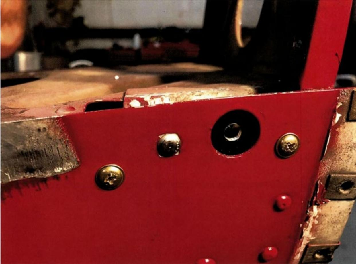
**Figure 35: View of finished Reinforcement Splice Installation**
