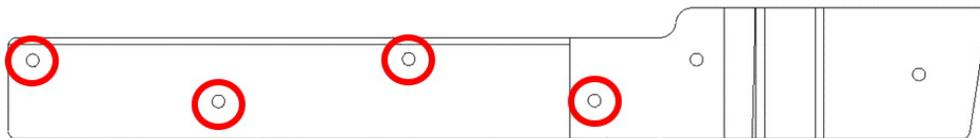
**Figure 17: Match Drill Diagram - #40 Bit**
