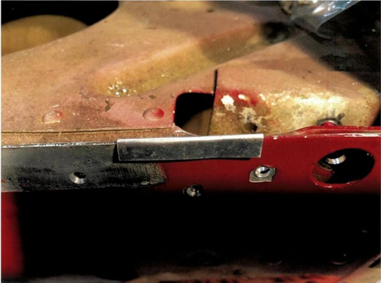
**Figure 10: Insert Guard between fuselage skin and reinforcement angle**
