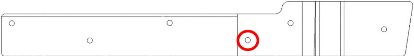
**Figure 23: Match Drill Diagram – Third Aft Hole**
