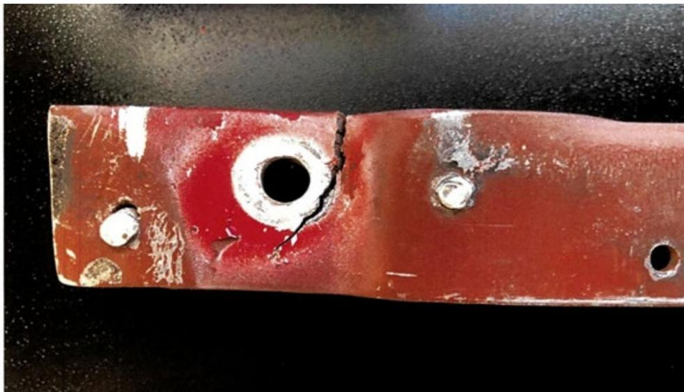
**Figure 3: Typical crack in the Tail Cone Reinforcement Angle (LH shown)**
