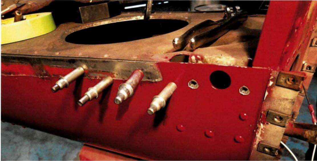
**Figure 18: Cleco Reinforcement Angle Splice onto aircraft**
