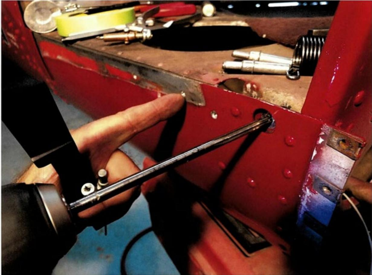
**Figure 7: Reaming Rear Pivot Holes**
