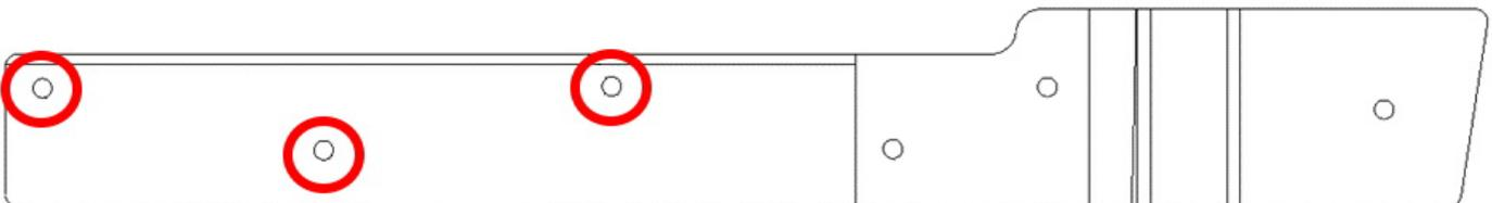
**Figure 24: Match Drill Diagram – Countersunk Rivet Holes**
