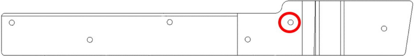
**Figure 22: Match Drill Diagram – Second Aft Hole**
