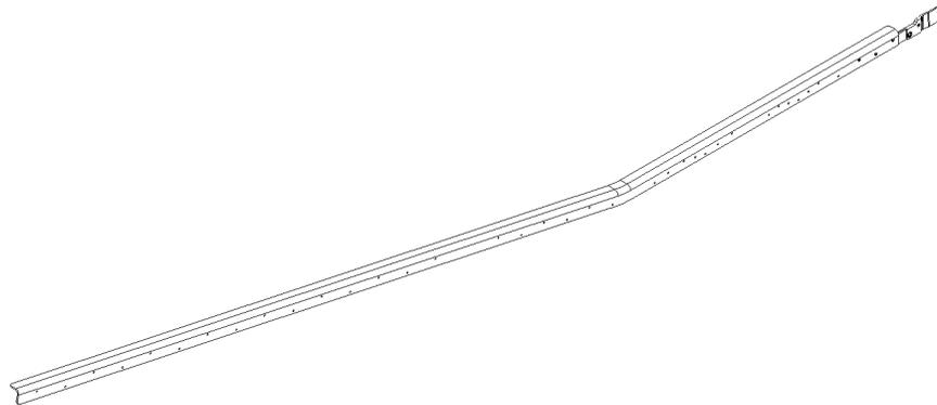
**Figure 4: STC design showing the Reinforcement Angle crack area replaced with STC reinforcement angle splice installed**
