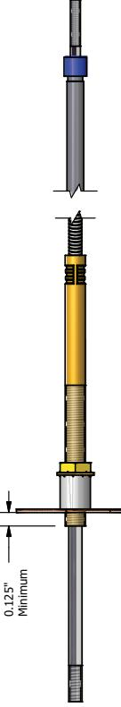
2. Carefully remove the jam nut from the retaining bolt on the panel bolt assembly.
