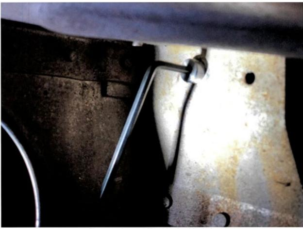
Figure 30: Insert drill guide shoulder bolt
