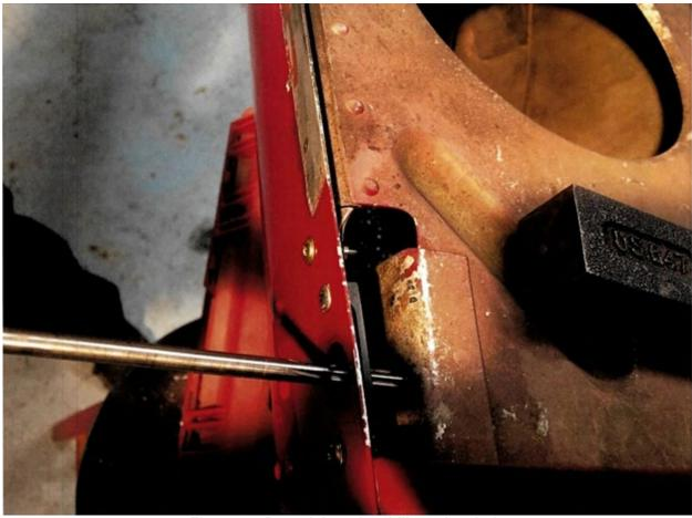
Figure 34: Ream inboard stabilizer pivot hole
