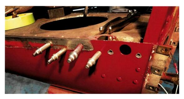
Figure 18: Cleco Reinforcement Angle Splice onto aircraft
