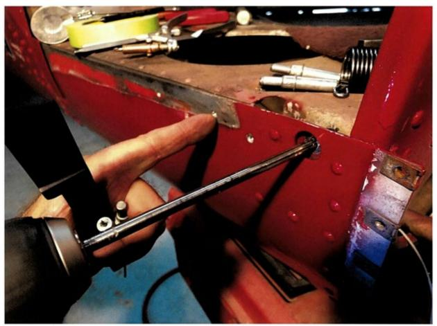
**Figure 7: Reaming Rear Pivot Holes**
