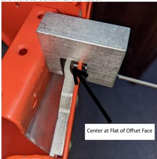
Figure 15: Drill Guide Assembly w/ Marking Pin
