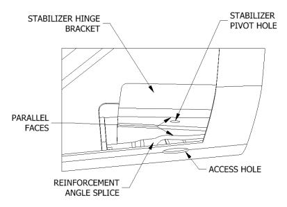
Figure 14: Reinforcement Splice Placement Diagram
