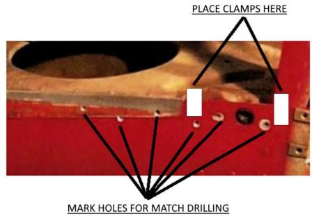
Figure 16: Hole Marking Diagram
