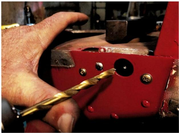
Figure 32: Open up pilot hole
