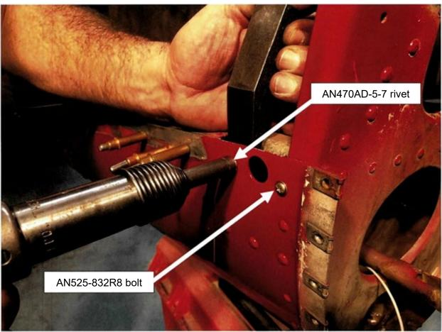
Figure 26: Rivet Reinforcement Angle Splice
