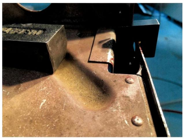
Figure 29: Insert drill guide assembly
