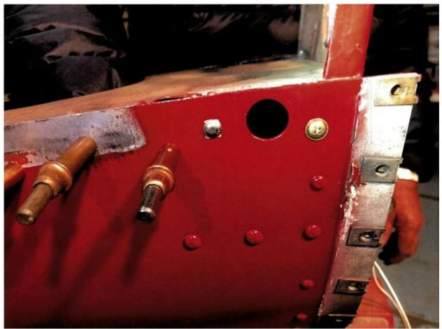
Figure 27: View after AN525-832R8 bolt and MS20470AD5-7 rivet installed
