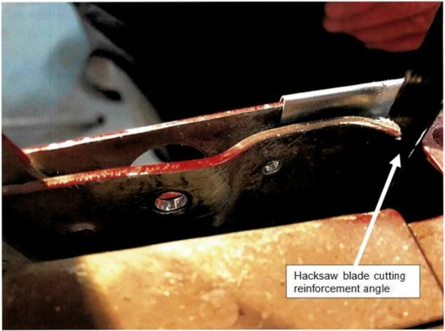
**Figure 11: Cutting Reinforcement Angle**
