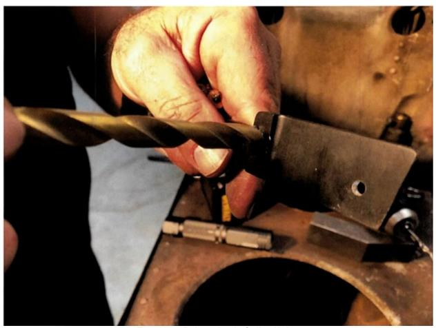
Figure 25: Deburr Angle Splice Holes
