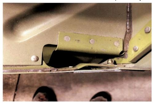
Figure 2: Tail Cone Reinforcement Angle (LH shown, RH opposite)
