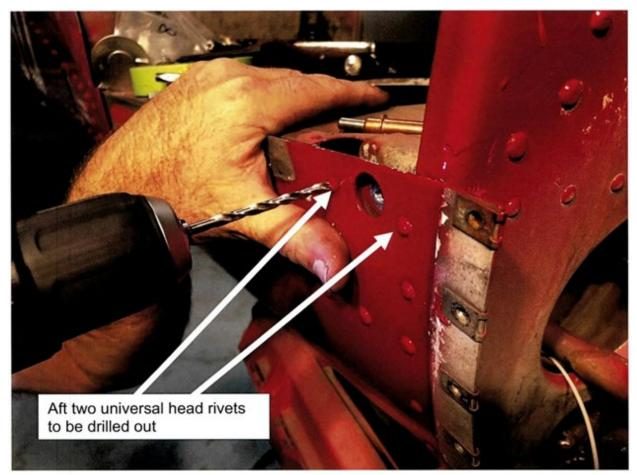
Figure 9: Drill out aft two AN470AD-4 rivets
