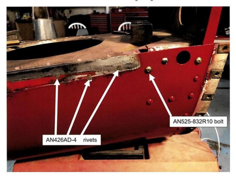
Figure 28: View after installing AN525-832R10 bolt and three MS20426AD4 flush head rivets
