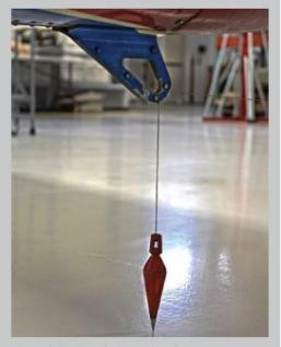
One of the hardest parts of proper rigging is determining where the nose tire is straight ahead.
